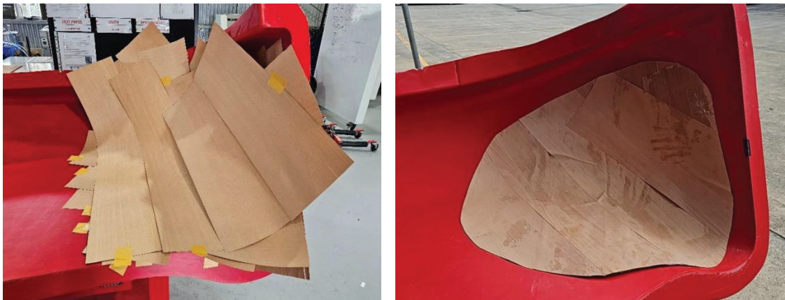
Figure 7. Section manufacture of the side of the panel with complex curvature showed the many relief cuts will be required but feasibility of full panel manufacture will be possible with methodical preforming and relief cuts prior to applying resin.
