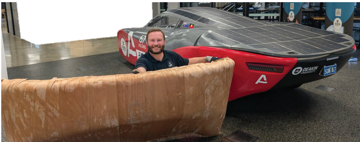
Figure 8. The full scale manufacture of the bumper panel proved that it is feasible to manufacture a large scale parge from wood veneers but requires different mould design and more research in to temperature and moisture control during forming, as detailed in Table 1.
