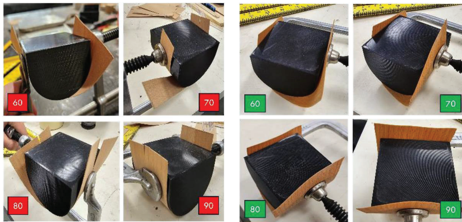
Figure 3. Comparison between bending the dry beech veneer around a 25 mm radius where it fails at 60° grain orientation and above (left), and the successful bending of the same set up when steamed for 60 seconds (right).
