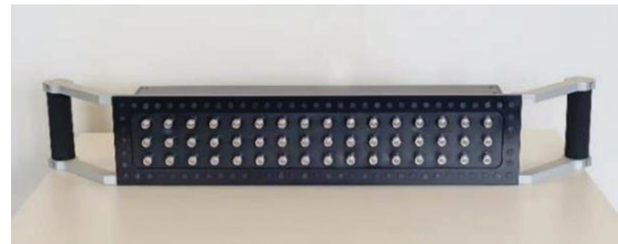
Figure 8. Newly developed ultrasonic array for cuboid test specimens (photo: MFPA, Martin Schickert)
