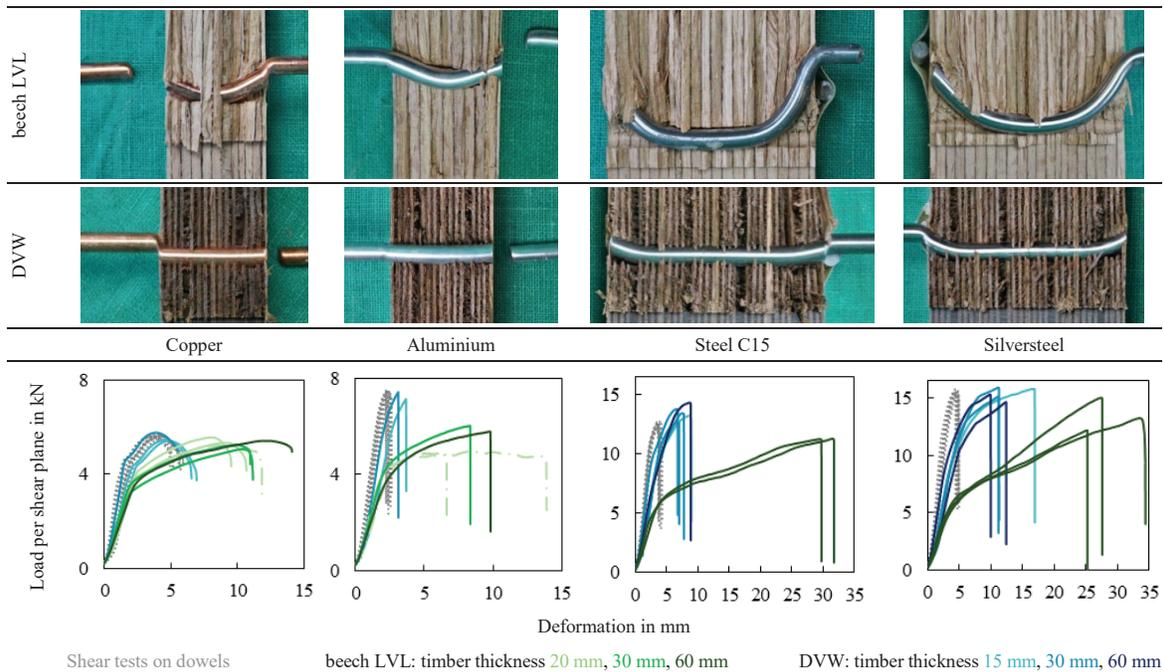
Figure 3: Deformed fasteners and failures for different dowels in beech LVL (1<sup>st</sup> line) and DVW (2<sup>nd</sup> line) with test results per shear plane below.
