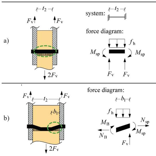
Figure 2: Force diagrams for two possible failure modes:
