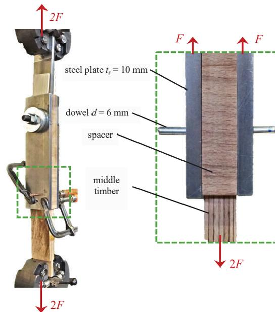
Figure 1: Test setup for connection tests.
