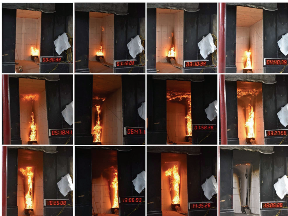
Figure 5: Images during Test 6 showing burner and clock with time in mm:ss.ms.
