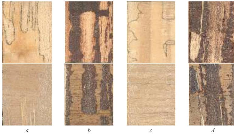
Figure 3. Typical failure modes of paired shear planes from 3-layer CLT panels made of *E. bosistoana* (*E*) and *radiata* pine (*P*) in the PEP configuration in block shear tests, using different adhesives: (a) MUF, (b) PRF, (c) PUR, and (d) RF.
