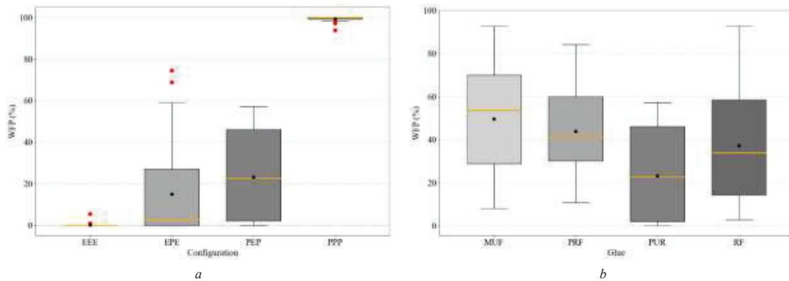
Figure 4. Comparison of WFP resulted from block shear test for the tested 3-layer CLT panels made of *E. bosistoana* (*E*) and *radiata* pine (*P*) with different configurations of EEE, EPE, PEP, and PPP (a) and in the PEP configuration with different adhesives of MUF, PRF, PUR, and RF (b).
