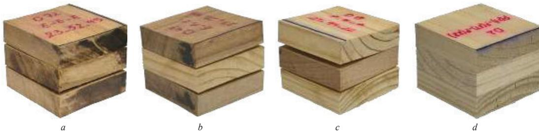
Figure 7. Representative delamination of 1C-PUR bonded *E. bosistoana* (E) and *radiata* pine (P) 3-layer CLT samples with different configurations: (a) EEE, (b) EPE, (c) PEP, and (d) PPP.
