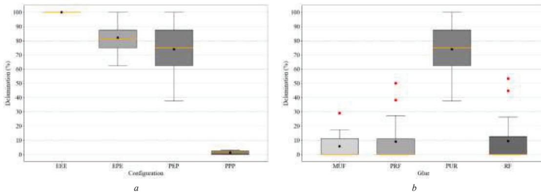
Figure 6. Comparison of DR resulted from delamination test for the tested 3-layer CLT panels made of *E. bosistoana* (E) and *radiata* pine (P) with different configurations of EEE, EPE, PEP, and PPP (a) and in the PEP configuration with different adhesives of MUF, PRF, PUR, and RF (b).
