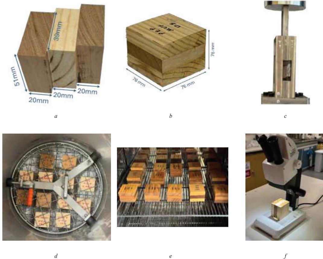
Figure 1. (a) block shear specimens, (b) delamination specimens, (c) shearing tool, (d) delamination specimens in the pressure vessel, (e) delamination specimens in the oven, (f) specimens under microscopic assessment.
