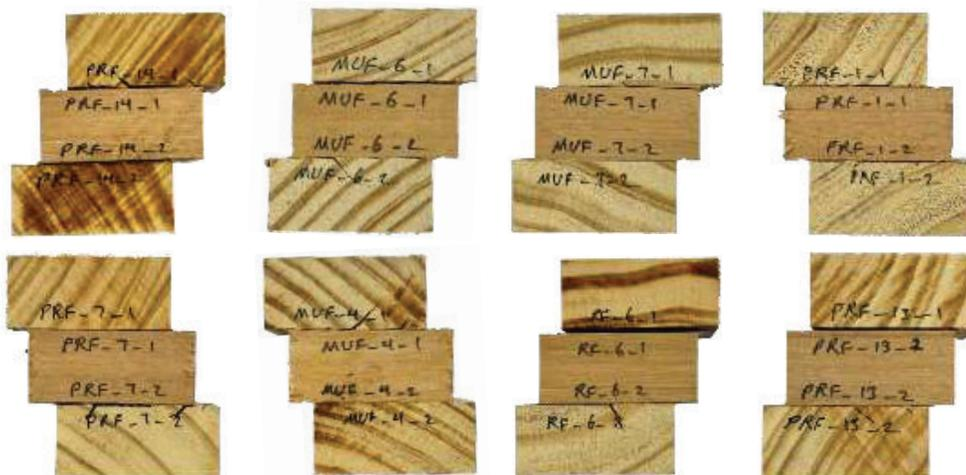
Figure 5. The ideal failure mode of mixed species CLT with the configuration of PEP under shear test bonded with PRF, MUF, and RF: perpendicular-to-grain shear failure of radiata pine.
