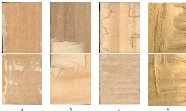
Figure 2. Typical failure mode of paired shear planes from 1C-PUR bonded *E. bosistoana* (E) and radiata pine (P) 3-layer CLT in block shear tests: a) EEE, b) EPE, c) PEP, and d) PPP.
