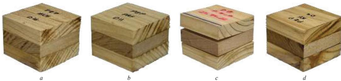
Figure 8. Representative delamination of 3-layer CLT panels made of *E. bosistoana* (E) and radiata pine (P) in the PEP configuration using different glues: (a) MUF, (b) PRF, (c) PUR, and (d) RF.
