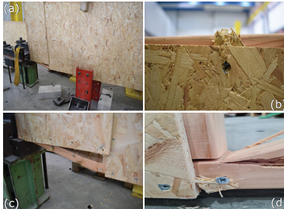
Figure 7: Pictures of the most common failure modes. (a) Failure located in the second-to-last stud; (b) Tearing of OSB; (c) Localized tearing of sheathing in the lower rail; and (d) Splitting underneath the second-to-last stud.
