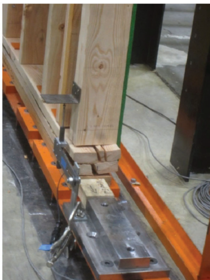
Figure 5: Typical cross-grain splitting caused by eccentricity between the one-sided WSP sheathing and the anchor bolts
