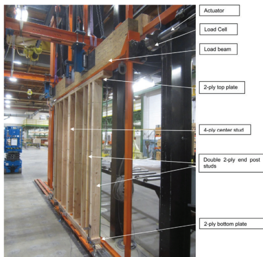
Figure 2: High-capacity shear wall test setup
