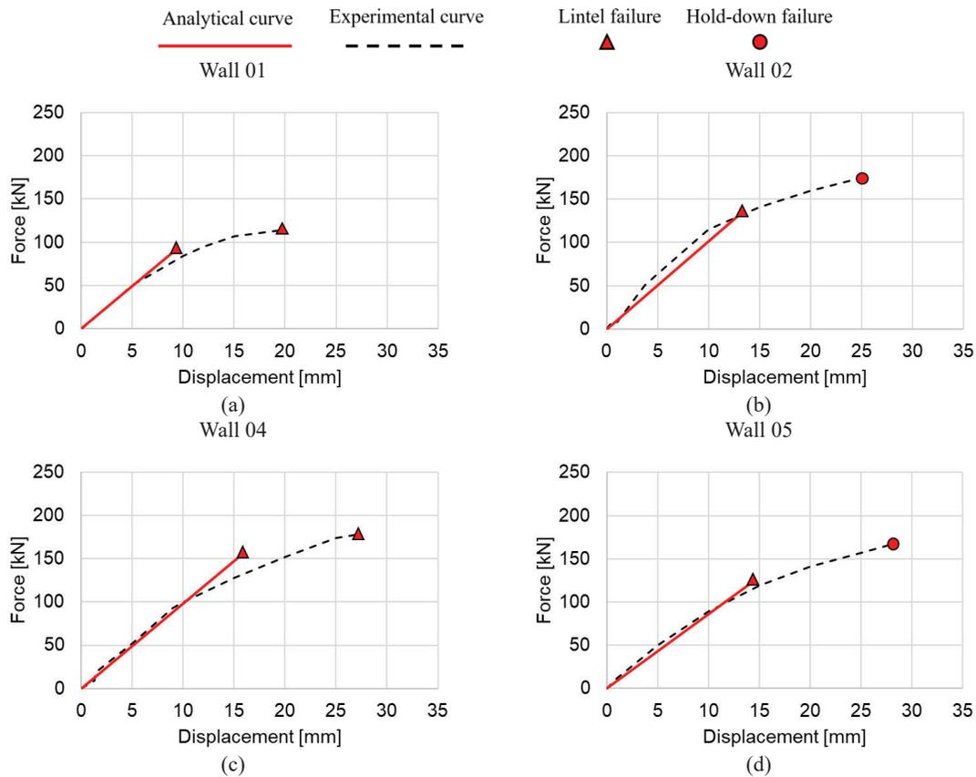
Figure 3. Comparison between the load–displacement curves of analytical model and experimental test.
