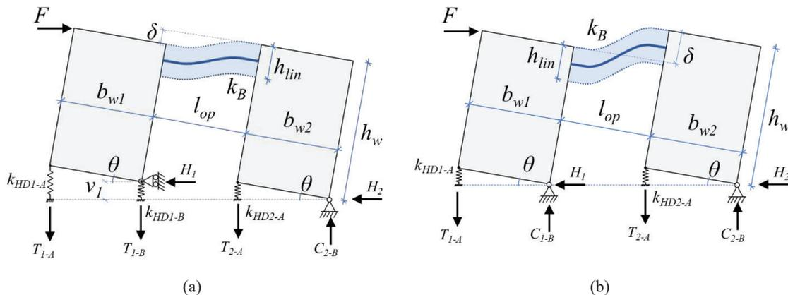
Figure 1. Analytical model: kinematic behaviour with one (a) and two (b) centres of rotation.
