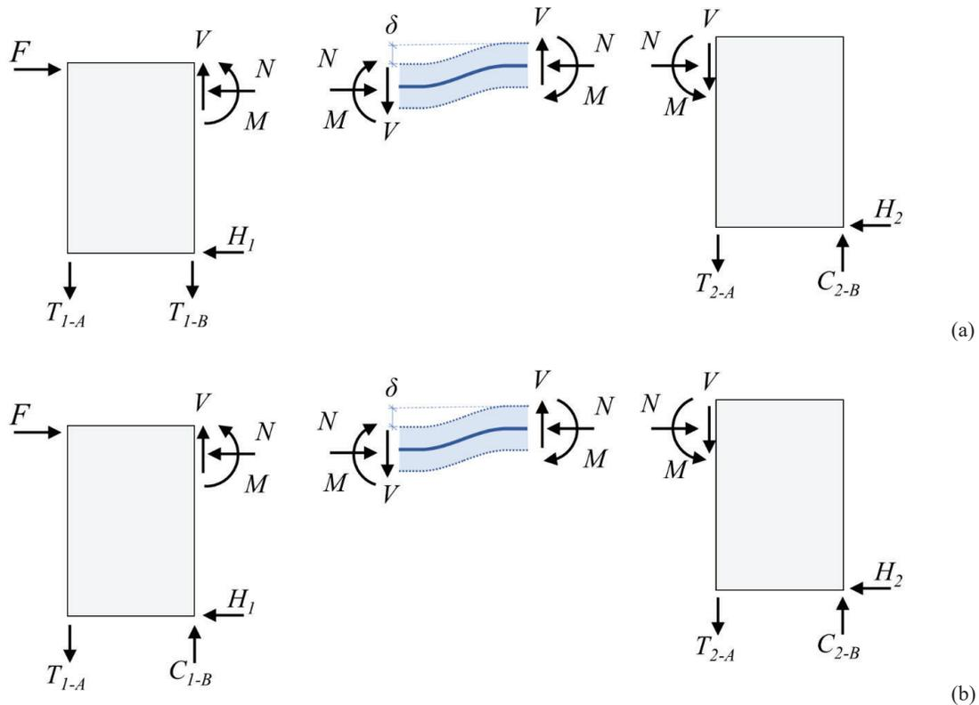
Figure 2. Internal and external forces in the wall segments and the lintel for the kinematic behaviour with one (a) and two (b) centres of rotation.
