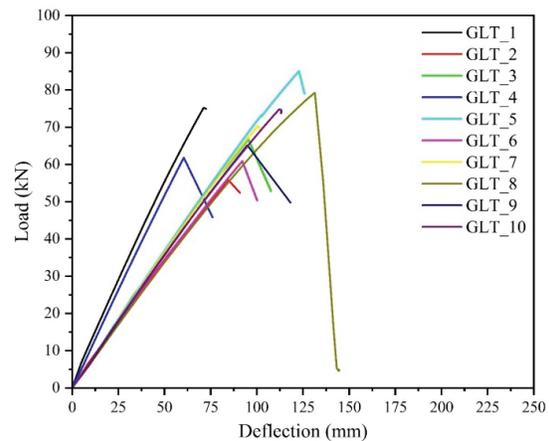
Figure 3: The load-deflection curves of glulam beams tested.
