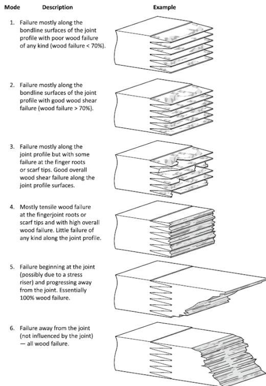
Figure 5: Classification of failure modes of finger-joint specimens referred from [25].
