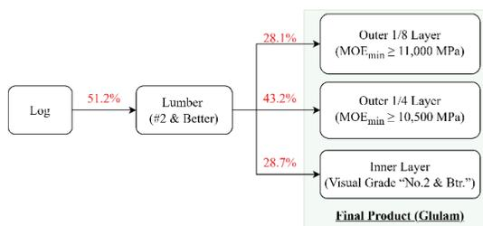
Figure 7: Estimation of the lumber yields for producing trembling aspen glulam beams.
