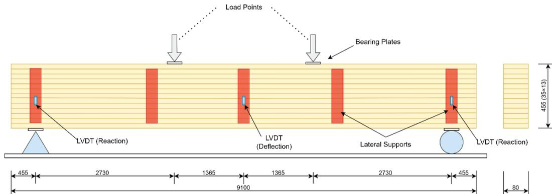
Figure 1: Schematic of testing a glulam beam under bending.
