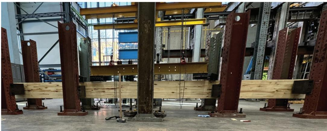
Figure 2: Setup for testing a glulam beam under bending.
