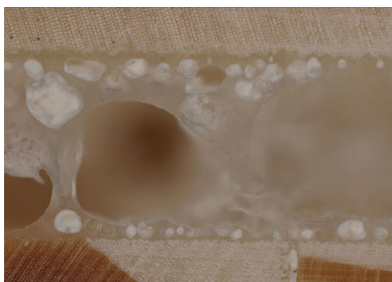
Figure 8. Bond line thickness at the position 44 mm and the configuration nails with a preload of 430 N; 50x magnification.
