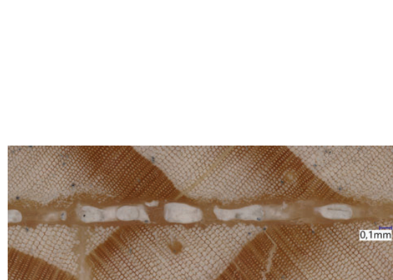
Figure 9. Bond line thickness at the position 1964 mm and the configuration staples with a preload of 740 N; 50x magnification.
