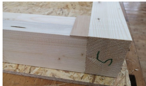
Figure 4. Part of the frame, where the cross beam was produced with a 2 mm protrude, represented using a 2 mm thick beechwood strip
