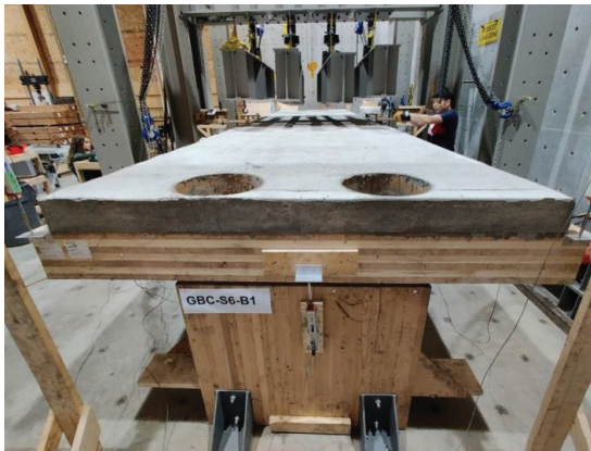
Figure 3. Lab test photo of the TCC slab band beam
