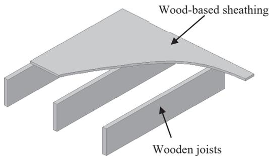
Figure 2: A typical wood floor system
