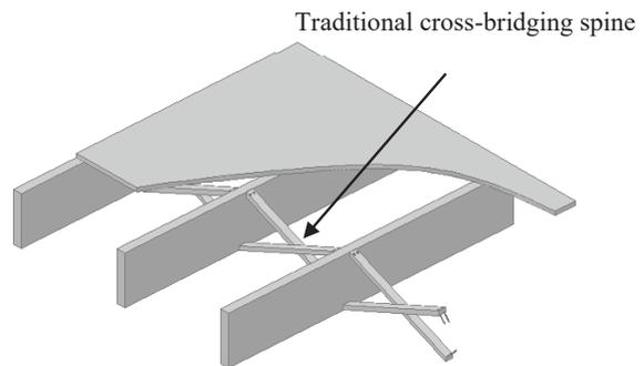
Figure 4: A wood floor with a row of traditional cross-bridging elements, connected by two nails with wood joists.
