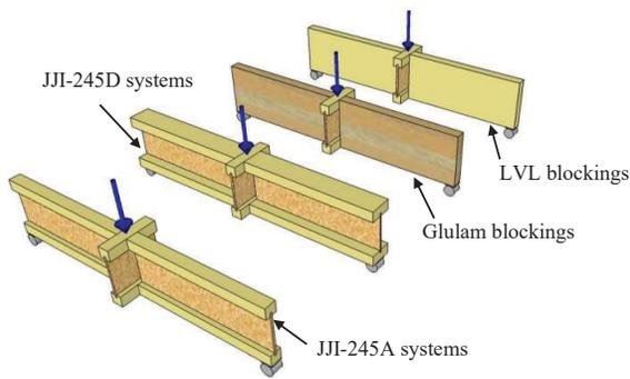
Figure 6: Typical blocking systems tested for bridging rotational stiffness
