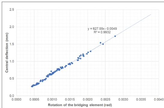
Figure 10: A comparison of the central deflection tested specimens and the rotation of the bridging elements at 75mm from the centre
