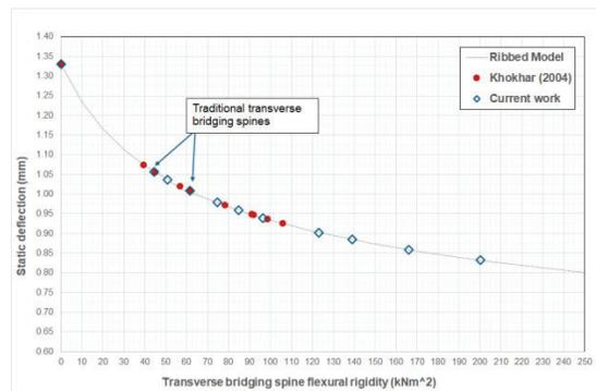
Figure 113: Influence of evaluated flexural rigidity of bridging spines on static deflection of a timber floor tested by Khokhar [].
