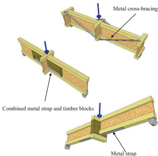
Figure 8: Typical hybrid bridging systems tested for the rotational stiffness
