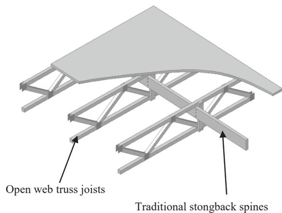
Figure 4: A wood floor with traditional strongbacks in open web truss joists.
