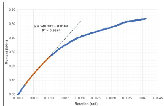
Figure 9: A typical moment and central rotation of bridging elements
