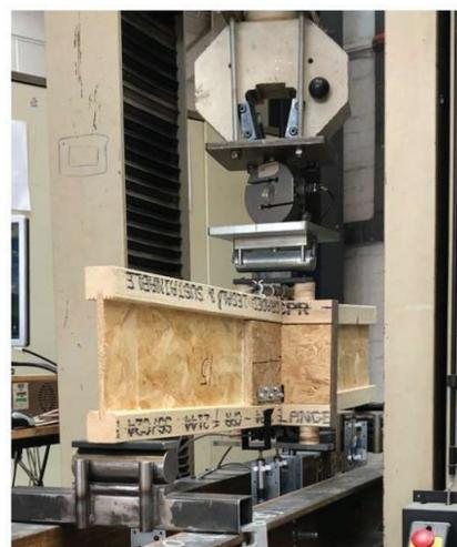
Figure 5: (a) A schematic diagram and (b) a typical single bridging element test setup
