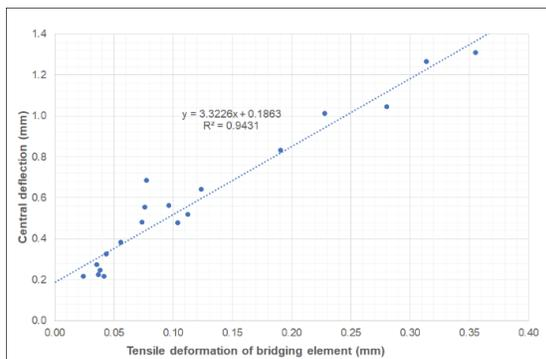
Figure 11: A correlation between the central deflection and compressive deformation of a bridging element
