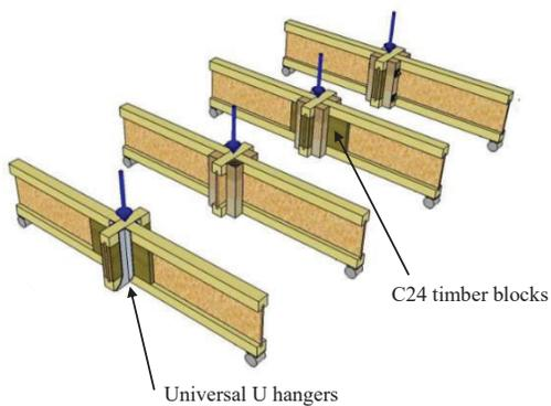
Figure 7: Typical blocking systems reinforced with steel hangers and timber wood blocks
