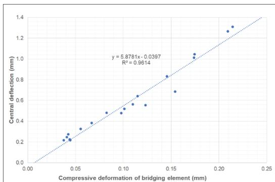
Figure 12: A correlation between the central deflection and tensile deformation of a bridging element
