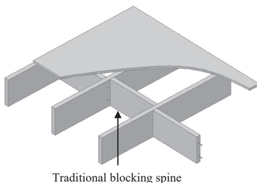
Figure 1: A wood floor with a row of traditional blocking elements connected by two nails with wood joists.
