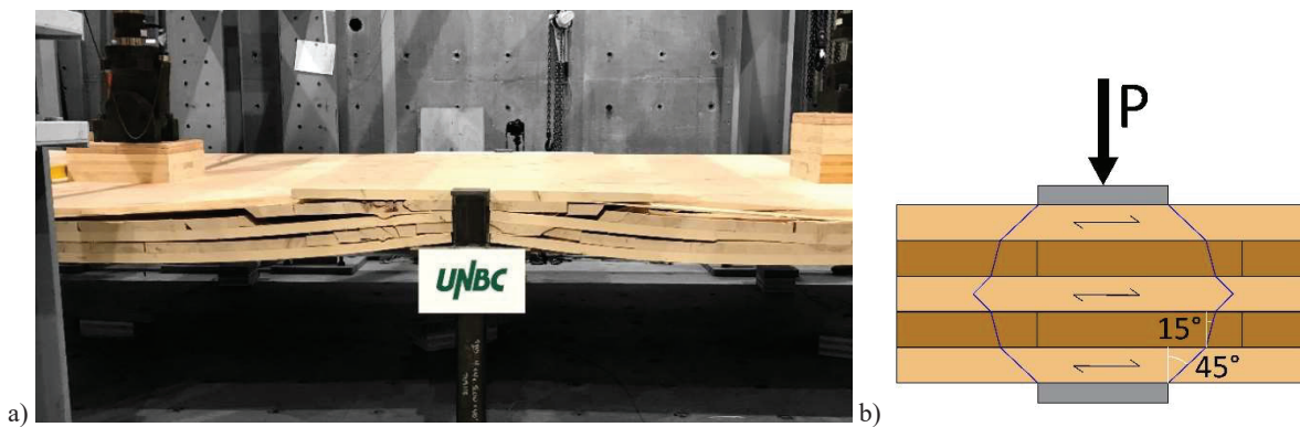
Figure 1. Point-supported CLT punching shear failure (a); CLT load dispersion model (b).
