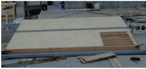
Figure 5. CUREE W-27 Test Details, Diaphragm with corner opening [3]
