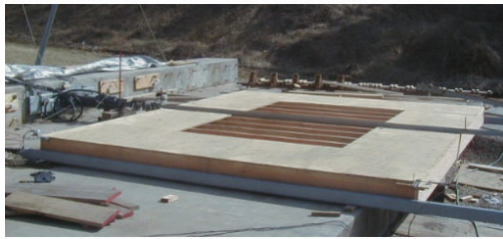
Figure 6. CUREE W-27 Test Details, Diaphragm with center opening [3]
