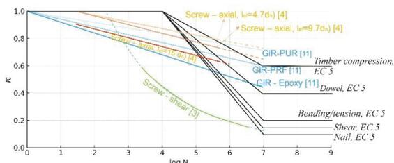
Figure 8. Comparison between testing results of different connections and provisions in EC5 at  $R=0.1$
