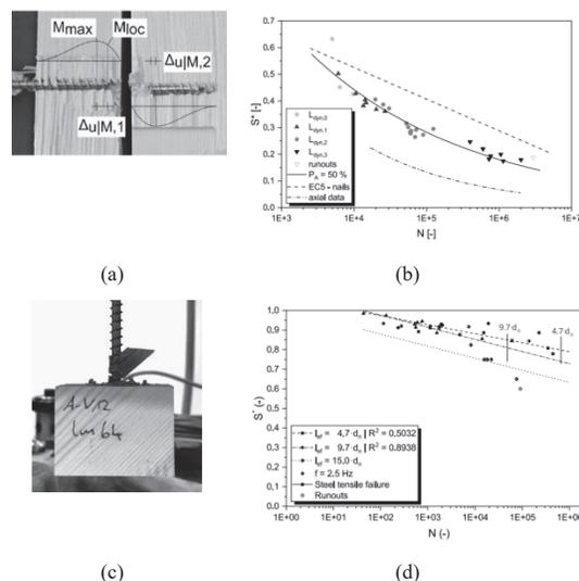
Figure 1. Fatigue testing on screws in shear and tensile directions [3][4]
