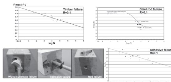
Figure 4. Fatigue behaviour of GiR and the associated S-N curve when designed for different kinds of failure [11]
