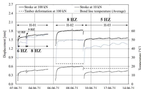
Figure 5. Temperatures in the bond lines as a function of time [14]
