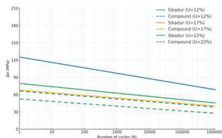
Figure 6. Fatigue performance of GiR under different moisture content (plotted according to [15])
