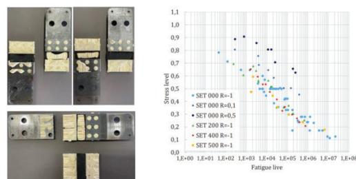
Figure 3. Fatigue testing on GiP connection [10]
