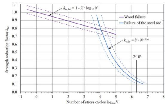
Figure 7. Fatigue strength reduction factor  $k_{fat}$  considering wood and steel failure [14]
