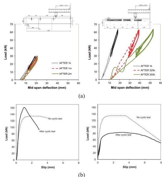
Figure 2. Comparative study on fatigue behaviour of rectangular notch floor beam (left) and metal plate floor beam (right): (a) stiffness reduction during fatigue testing; (b) post fatigue behaviour.
