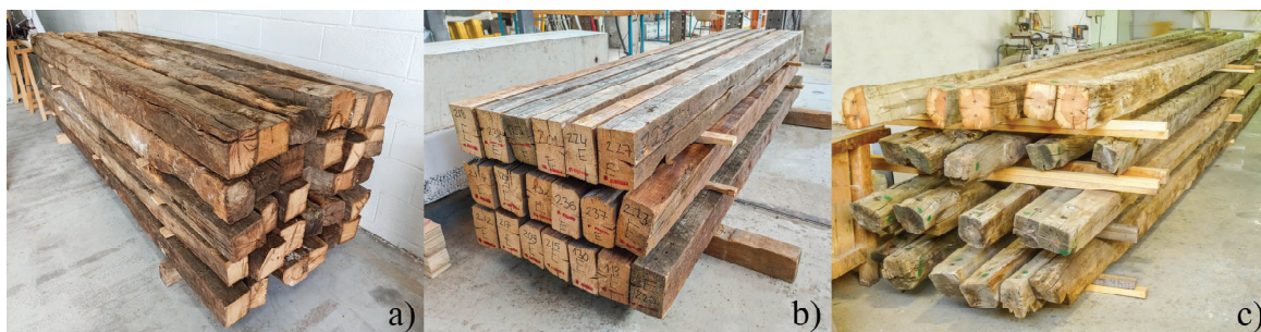
Figure 1. a) European oak specimens from InFutUReWood project b) Norway spruce specimens from RECOWERS project c) Salzmann pine specimens from BIA 2014-55089-P project.
