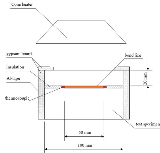
Figure 5 Test specimen setup under the cone heater.
