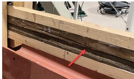
Figure 8 Insufficient contact surface between the lamellae.
