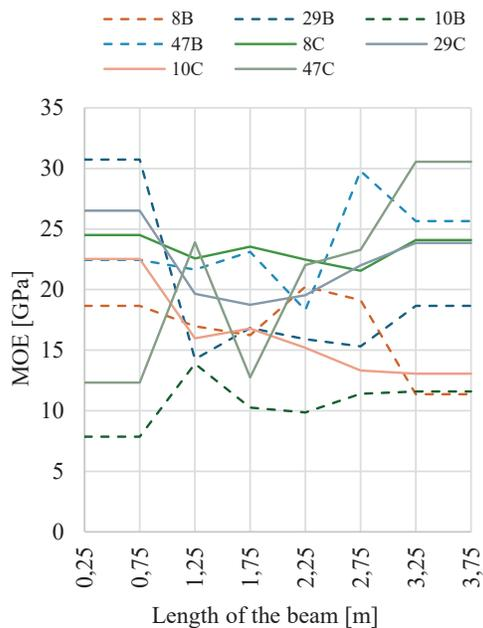
Figure 6 Stiffness values of the SBI-PUR beam lamellae.
