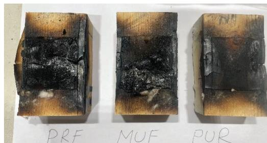
Figure 10 Specimens after fire test of bond line.
