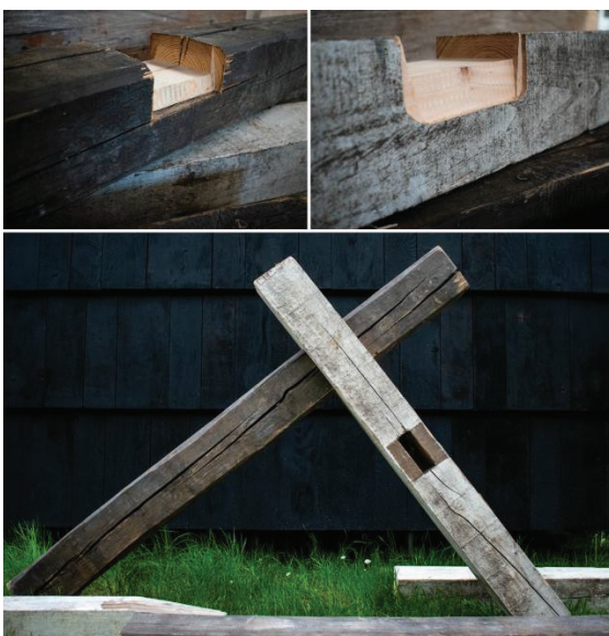
Figure 10. Fabricated timber joints and joined partial structure
