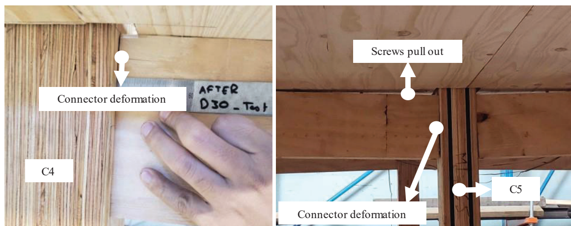
Figure 4. Deformation of the substructure after Test D30
