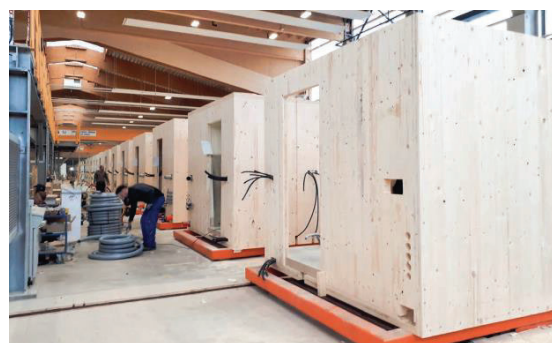
Figure 3. Volumetric modular elements in factory
