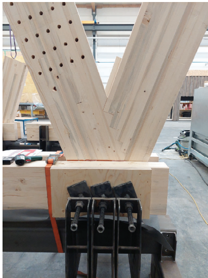
Figure 7. Manufacturing of glued truss node test specimens
