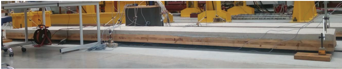
Figure 1. Prestressed CLT-concrete composite panel after anchor removal with visible camber.
