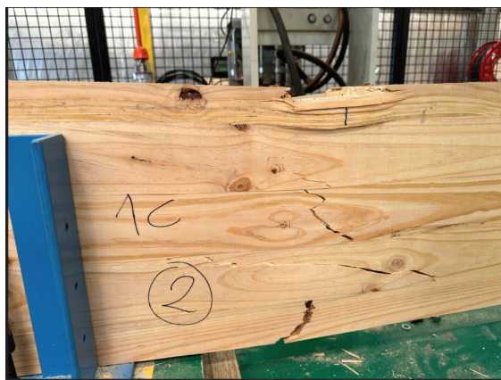
Figure 13 – Set 1C sample showing shear failure
