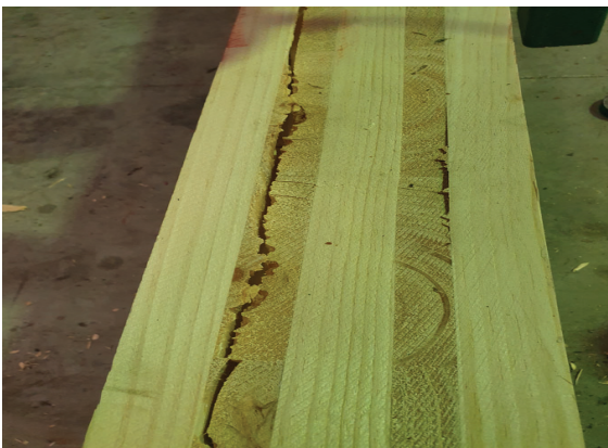
Figure 8 – CL5/140 x 330 deep beam (18×D) sample with cracking in internal lamella
