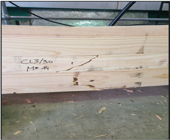
Figure 7 – Typical being failure in bending tests
