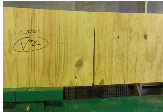
Figure 9 – Typical failure mode in CL3/90 x 450 deep beam (8×D) sample with vertical outer lamellas
