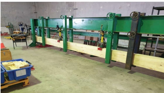
Figure 6 – 4-point bend test set up
