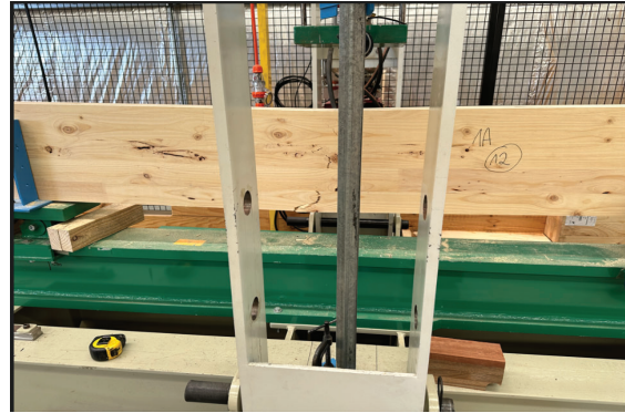
Figure 11 – Set 1A sample showing bending failure near mid span
