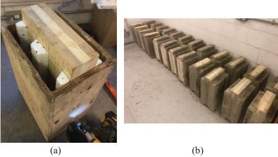
Figure 2: (a) CLT Specimen with attached EPS panels and screws in formwork and (b) CLT-concrete composites
