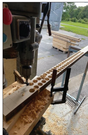
Figure 1. Preparation of lamellae for prototype 4 (22 mm holes)
