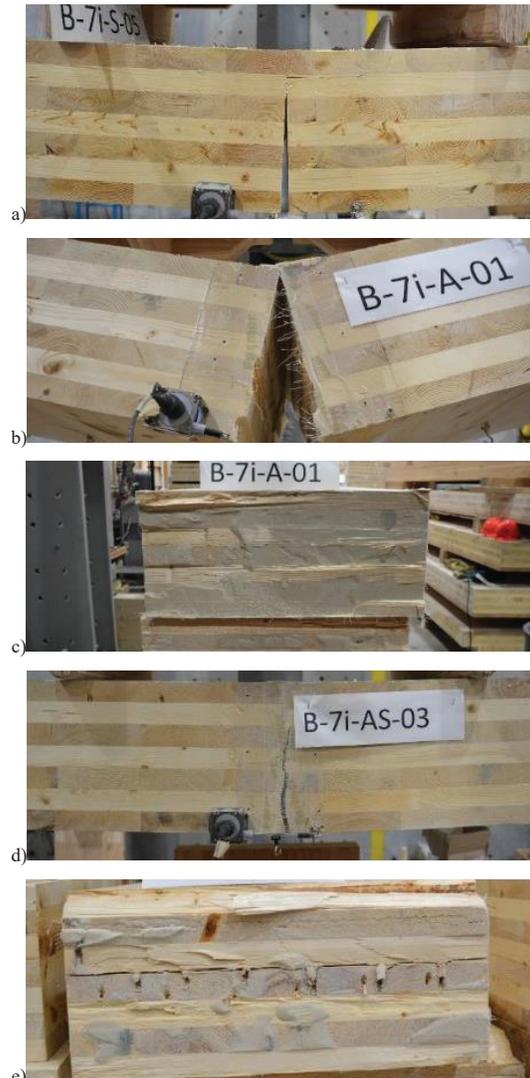
Figure 4. Typical failure modes in four-point bending tests.
