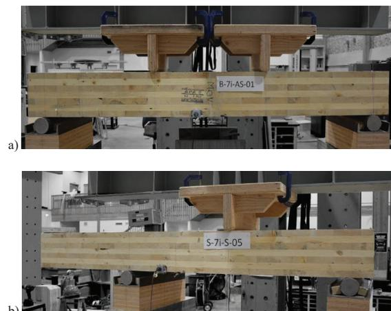
Figure 2. Test setup: a) four-point bending; b) three-point bending.
