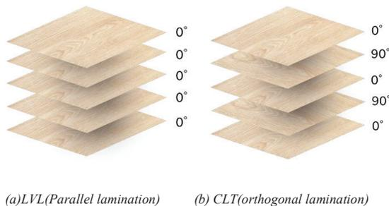
Figure 2. Conventional Laminated Timber Plates: (a) LVL (parallel lamination); (b) CLT (orthogonal lamination)
