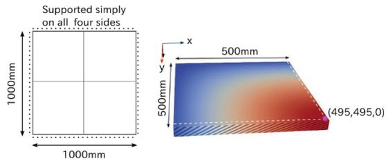
Figure 4. Numerical model Multi-Angle Laminated Timber (MALT) Model
