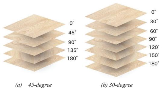
Figure 1. Multi-Angled Timber Plate Models: (a) 45-degree rotation; (b) 30-degree rotation
