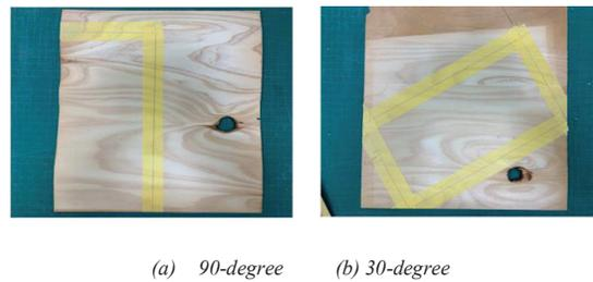
Figure 3. Material Preparation for Experimental Testing: (a) 90-degree orientation; (b) 30-degree orientation
