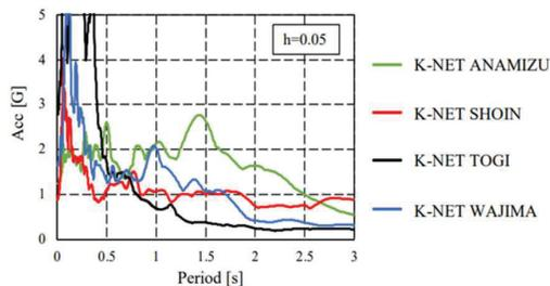
Figure 7. Acceleration response spectra
