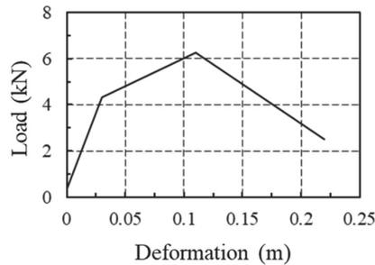
Figure 4. Restoring force behaviour of brace
