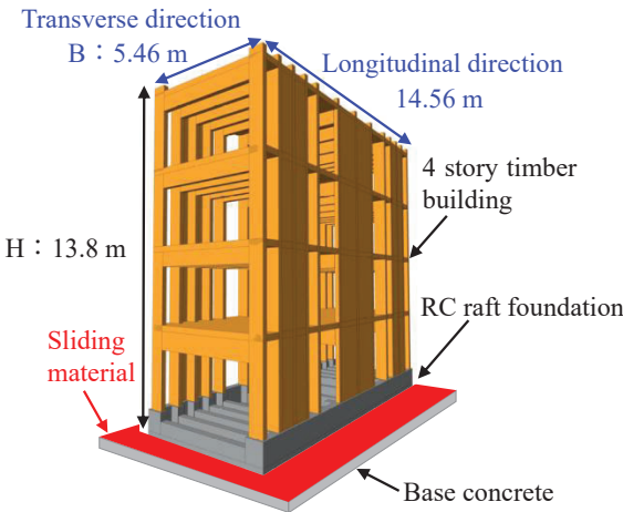
Figure 3. Four-story timber building with sliding base system
