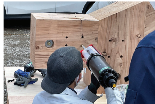
Mock-up of adhesive injection
