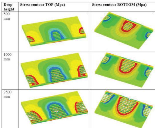
Figure 13. Top and bottom surface axial stresses on the CLT panel for different drop heights tests
