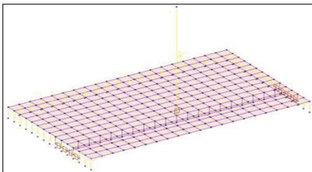
Figure 10. Detail of the DESK60 top panel in the numerical model
