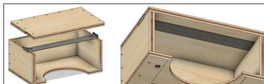
Figure 1. Steel reinforcement plate under the top panel of the desk
