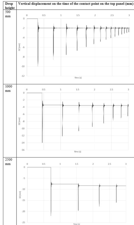
Figure 15. Impact point deflection on the CLT panel for different drop heights tests
