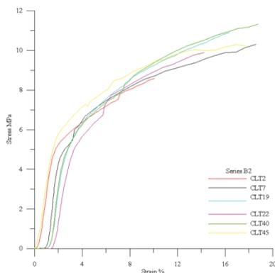
Figure 6. Stress-strain diagram of a CLT element compressed in direction parallel to the grain.
