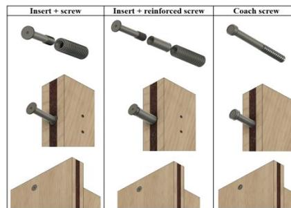
Figure 4. Types of connections analyzed
