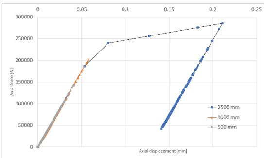
Figure 14. Axial force-displacement plot of the steel plate for different drop heights tests
