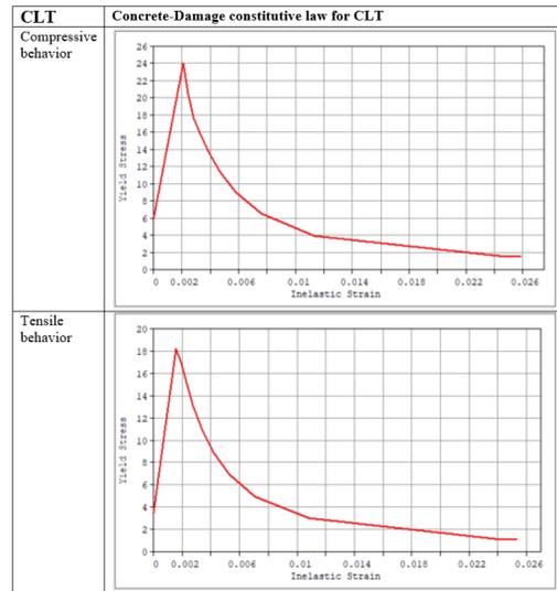
Figure 11. Concrete-Damage constitutive law for CLT (N/mm<sup>2</sup>)
