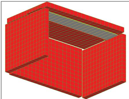
Figure 9. DESK60 numerical model (bottom view)
