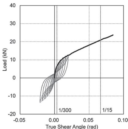
Figure 3 Load – true shear angle relationship of the NLT test specimens.
