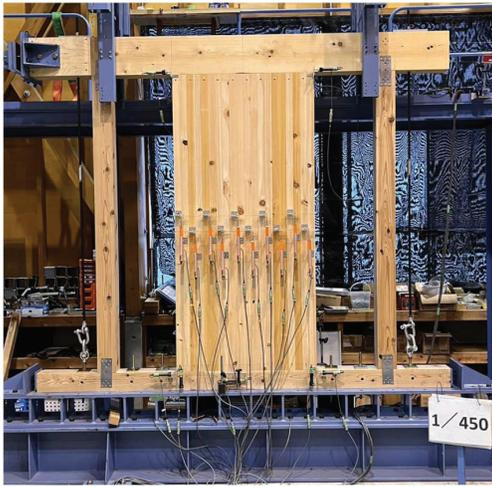
Photo 1 In-plane shear test
