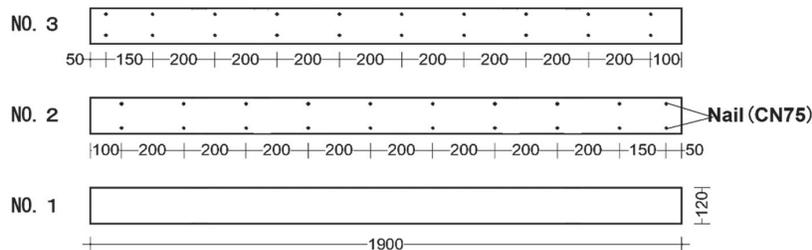
Figure.2 Location of the notches for the nail joints at the lumbers composing NLT.
