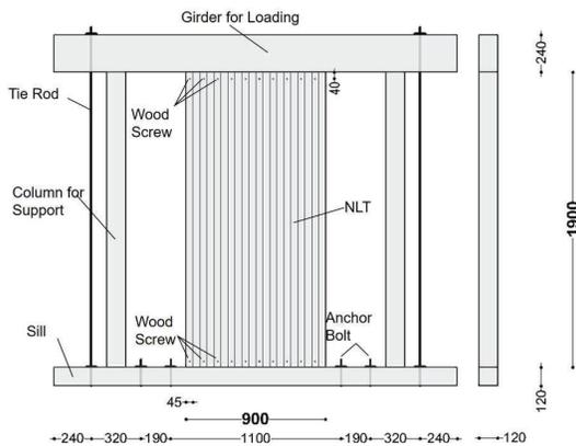
Figure.1 Assembly of the test specimens.
