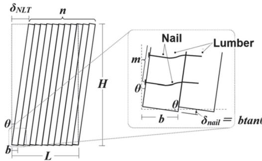
Figure 4 Modeling of Nail Joints of NLT
