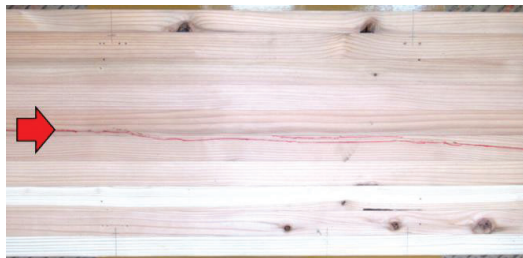
Figure 11: Failure of LSB specimen.
