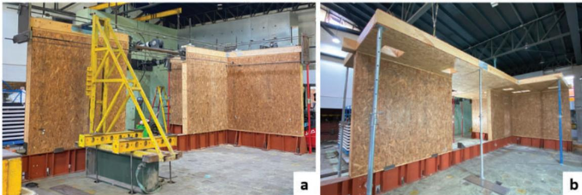
Figure 1. General configuration of the tested assemblies to evaluate the impact of: (a) TSW effect only; and (b) TSW effect + FDIA and AXL effects.
