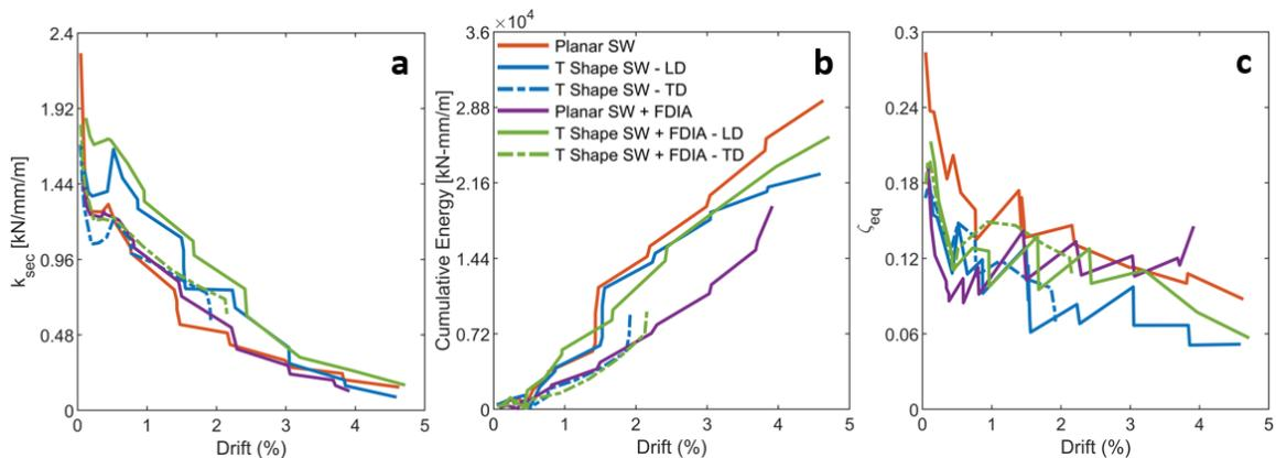
Figure 3. Comparisons between the (a) secant stiffness, (b) cumulative dissipated energy, and (c) equivalent viscous damping of the Planar SW and the T shape SW with different effects.
