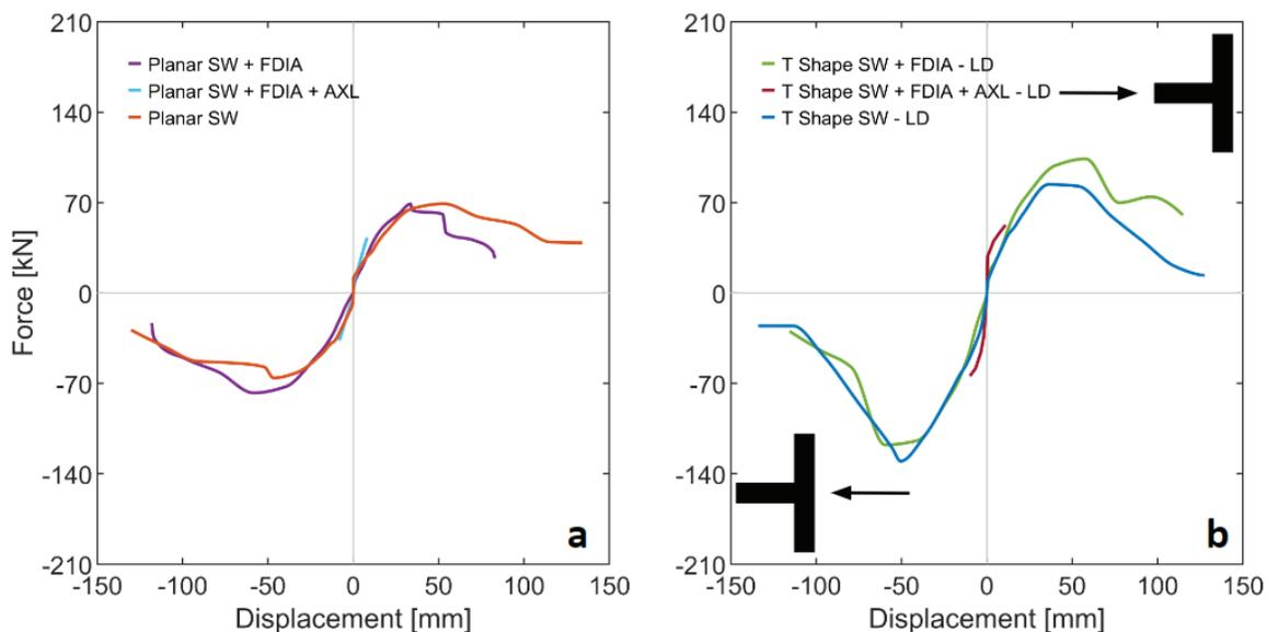
Figure 2. Backbone curves (longitudinal direction) of: (a) a Planar SW; and (b) a T-Shape SW.
