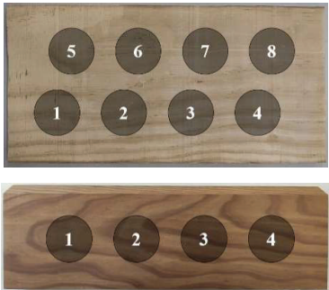
Figure 2. Points on the samples for colour analysis. (top) acetylated wood (Bottom) thermo-treated wood.
