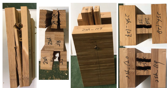
Fig. 17 Destruction property(Double Shear test(GLB))
