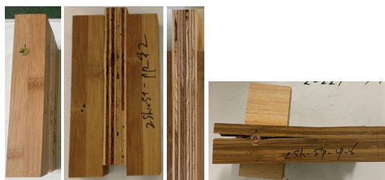
Fig. 18 Destruction property (Double Shear test(Plywood))
