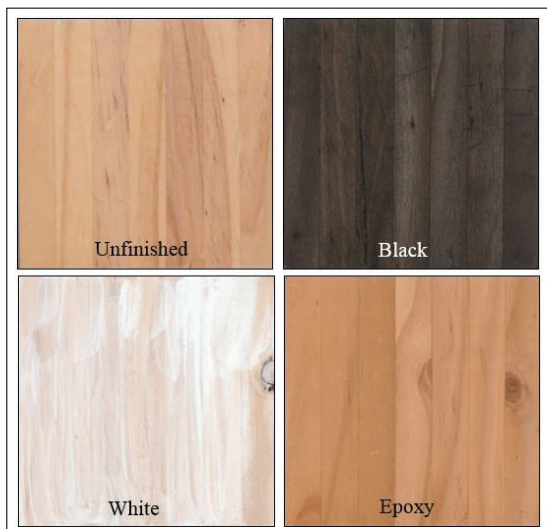
Figure 2. Radiata pine beam surfaces following the application of finish products.
