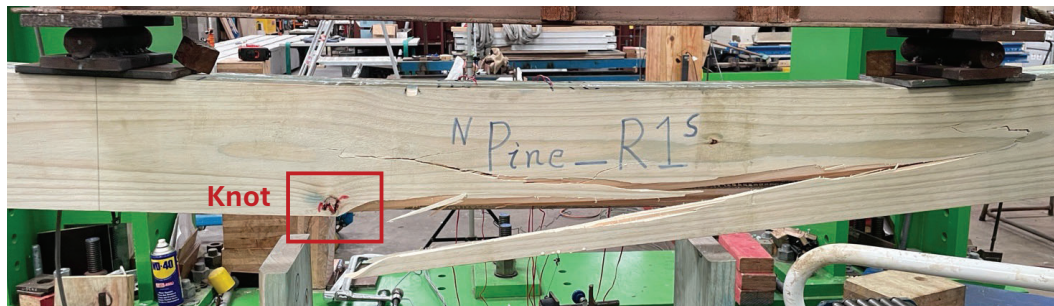
Figure 4. Example of failure mode for short-term beams.
