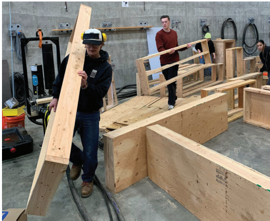
Figure 2. Fabrication of stressed-skin panels
