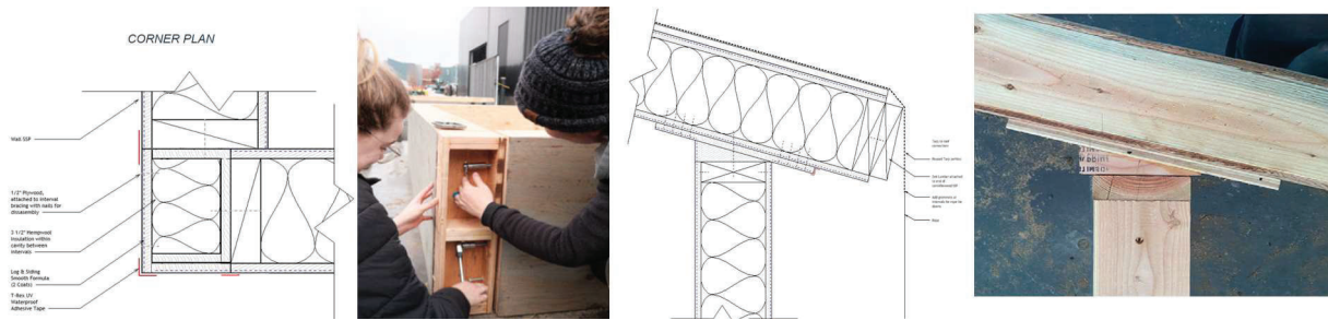
Figure 10. C-shaped connector boxes for corner connections (two images on the left). Roof connection (two images on the right)
