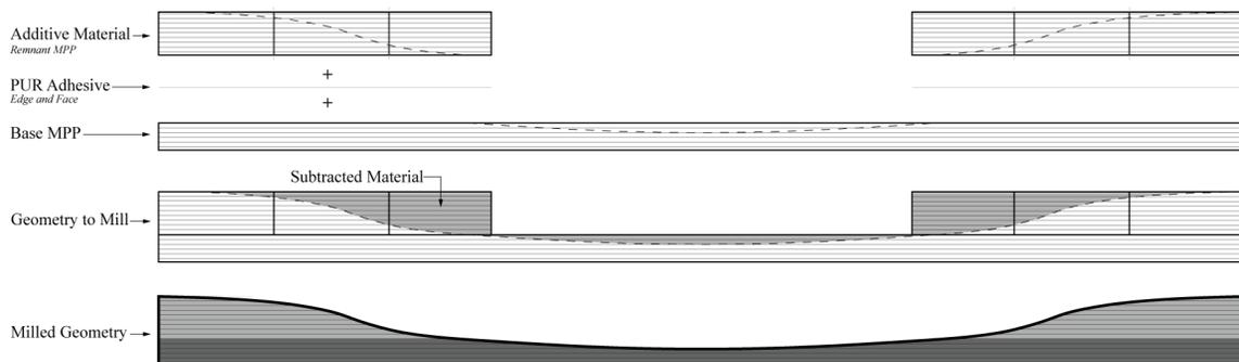
Figure 2. Sectional view example of additive fabrication
