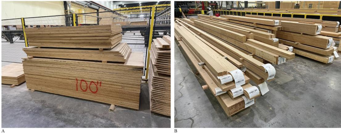
Figure 1. A: panelised MPP remnant material type B: rectilinear MPP remnant material type
