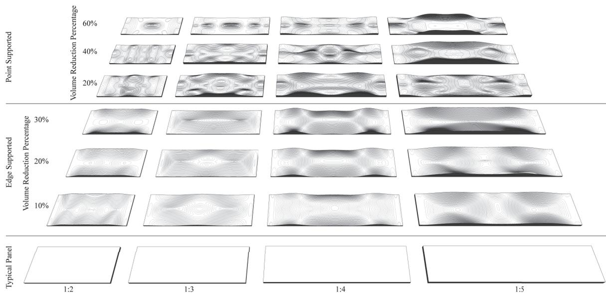
Figure 7. Example of design solution space with samples of edge and point supported optimization cases at incremental volume reduction percentages. The panel geometry is flipped to show the thickness throughout the panel.
