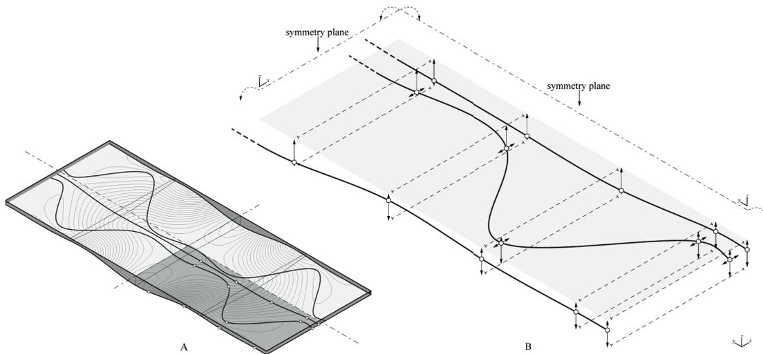
Figure 4. Constructed geometry and shaping model. A: surface lofting through mirrored curves to construct geometry with quadrant darkened. B: shaping model point position variable bounds and curve interpolation within quadrant.
