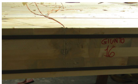
Figure 3. Thermocouples inside the joint
