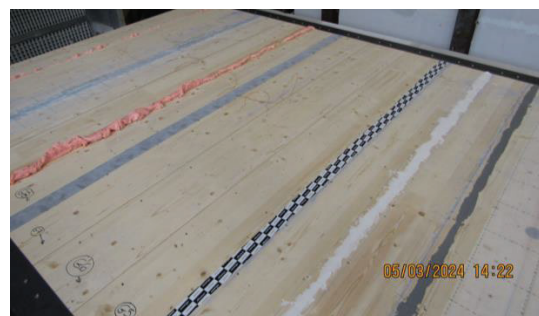
Figure 5. CLT slab (120mm) ready for testing
