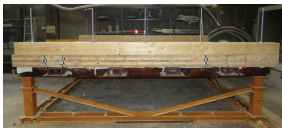
Figure 2. CLT slab (200mm) ready for testing
