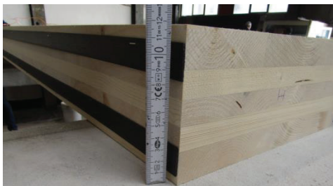
Figure 14. Fire stripe graphite installed in 8mm gap
