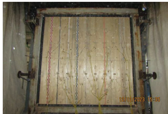
Figure 4. CLT wall (100mm) ready for testing
