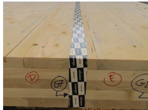
Figure 8. Flexi Band tape applied on the upper side
