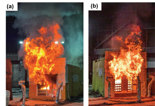
Figure 3. Photos of compartment fire tests (a) Test #2 (fully exposed mass timber with furniture) (b) Test #4 (full encapsulated mass timber with wood cribs)
