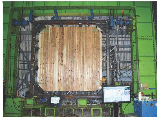
Figure 10. Shear wall test process
