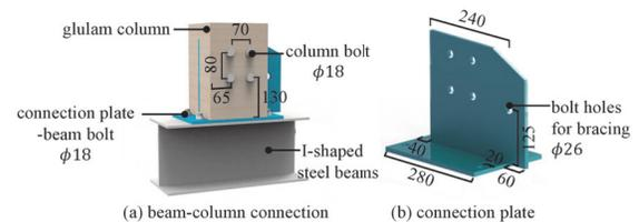
Fig. 4 Beam-column connection design
