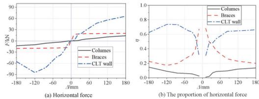
Fig.12 Horizontal force distribution of specimen F1
