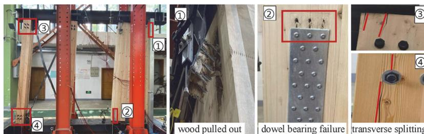
Fig.9 Failure mode of specimen F1
