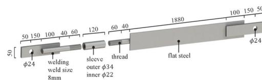
Fig. 5 Design of tension-only bracing
