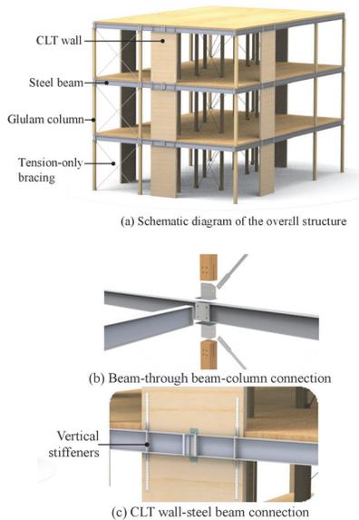
Fig. 1 Diagrams of beam-through steel-timber hybrid structures
