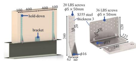
Fig. 3 CLT connections design
