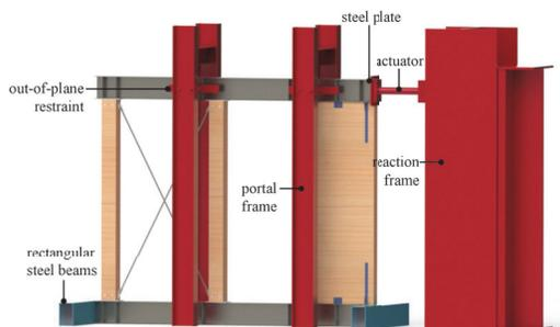
Fig.6 Loading schematic diagram
