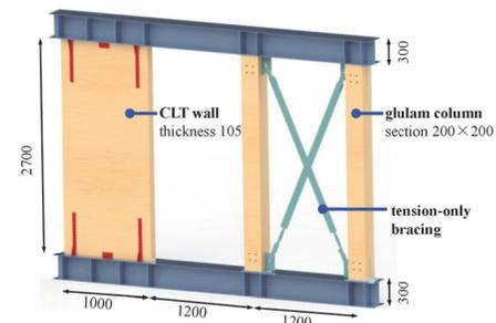
Fig. 2 Dimensions of the specimen
