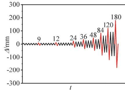
Fig.7 CUREE displacement loading system
