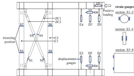
Fig.8 Layout diagram of measurements
