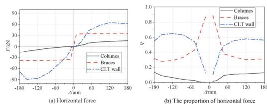
Fig.13 Horizontal force distribution of specimen F2
