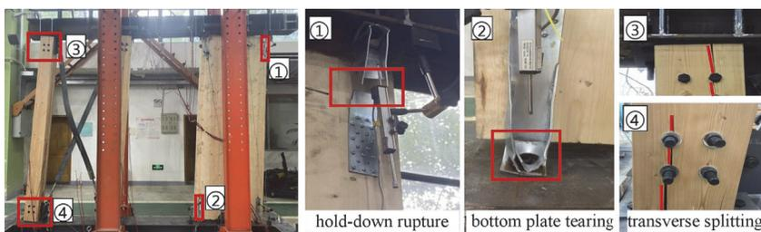
Fig.10 Failure mode of specimen F2
