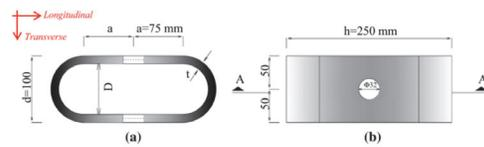
Figure 4: Steel cushions used as energy dissipators between the CLT panels, placed vertically at the panel-to-panel intersection, modified from [8]
