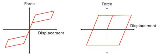
Figure 6: Example elastic-perfectly plastic (left) and flag-shaped (right) nonlinear spring response used for modelling the zero-length elements
