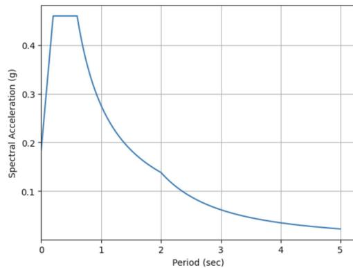
Figure 3: Design acceleration response spectrum
