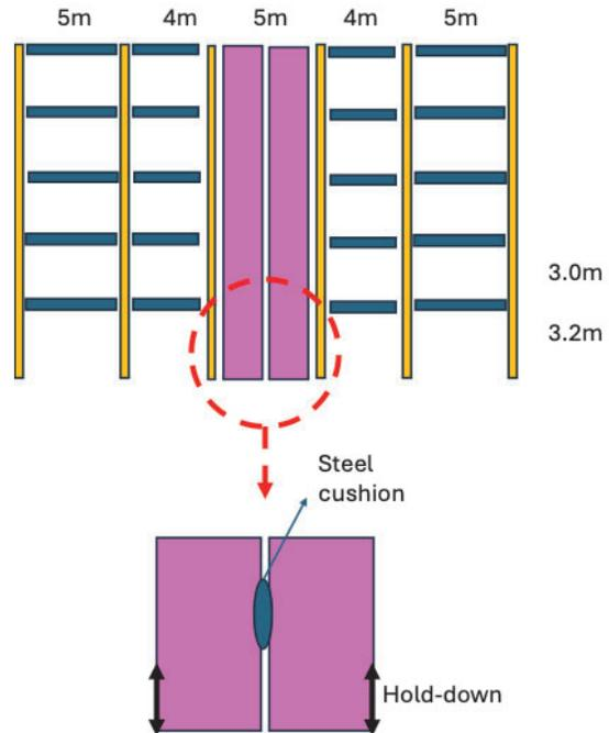
Figure 2: Section view of one of the lateral load bearing frames of the designed structure
