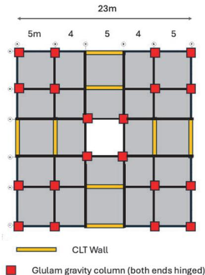
Figure 1: Plan view of the designed structure
