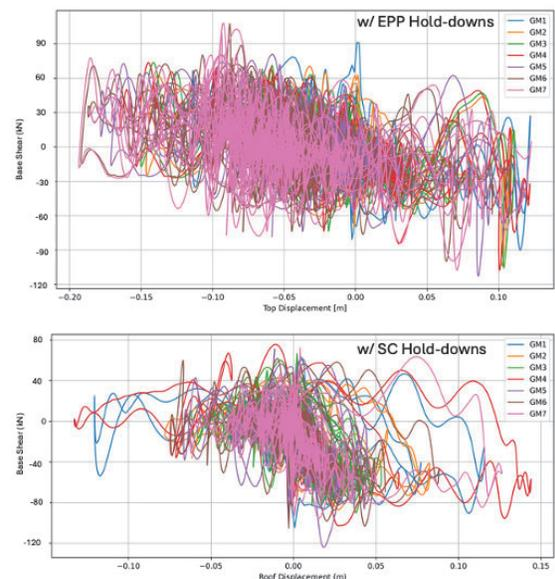
Figure 7: Roof displacement vs base shear plots from 7 records for the self-centering (top) and elastic-perfectly-plastic (bottom) hold-down configurations
