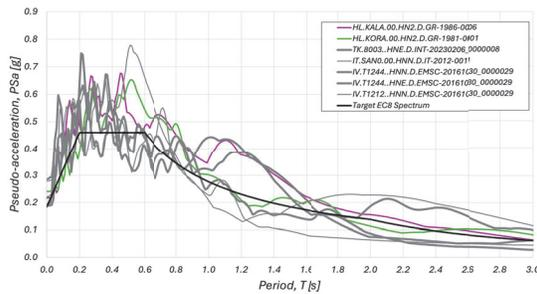
Figure 5: Acceleration design spectrum versus the selected records for Design Option 1,  $T_1=0.35s$  (above) and Design Option 2,  $T_1=0.50s$  (below)
