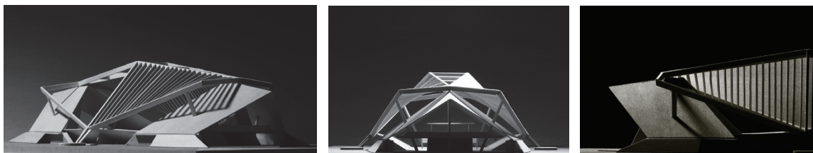
Figure 9 (a-c). A gymnasium with dual membrane roof supported by closed section rafters (Figure 4, B) used for solar energy collector.
