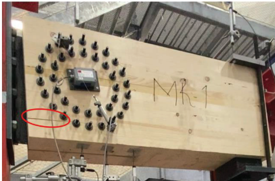
Figure 8: Final failure of the MR-1 specimen due to a tensile crack perpendicular to the grain of the timber.
