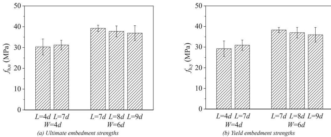
Figure 6. Embedment strengths of the specimens using smooth steel dowels with different loaded end distances
