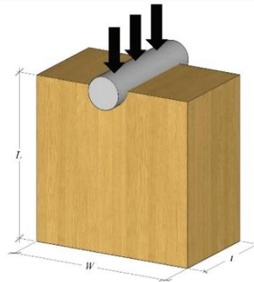
Figure 2. Dimensions of embedment specimen
