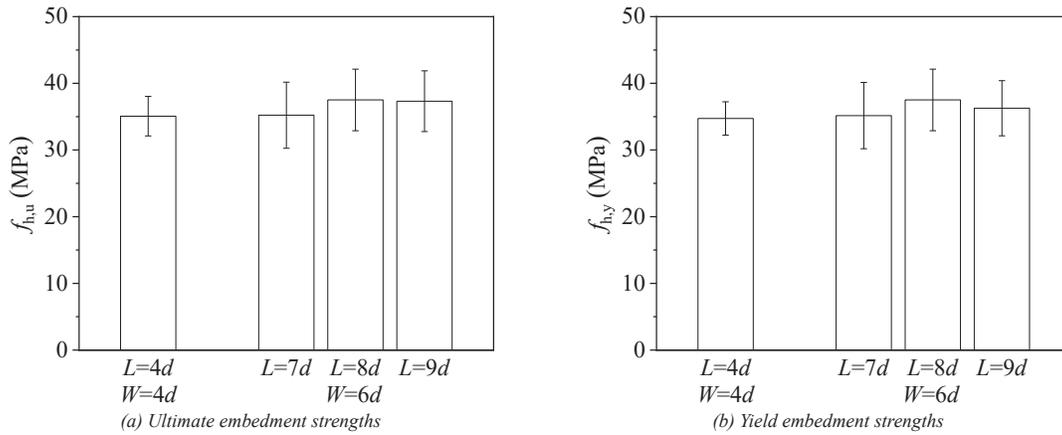
Figure 7. Embedment strengths of the specimens using DW dowels with different loaded end and edge distances
