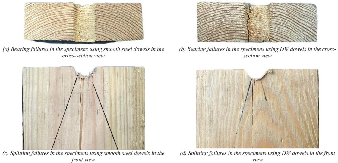
Figure 5. Failure modes in the specimens
