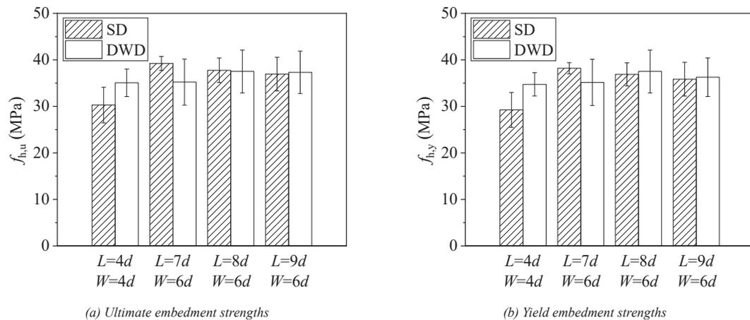
Figure 9. Embedment strengths of the specimens using smooth steel dowels and DW dowels
