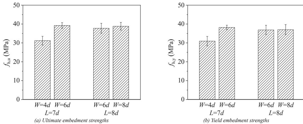
Figure 8. Embedment strengths of the specimens using smooth steel dowels with different edge distances
