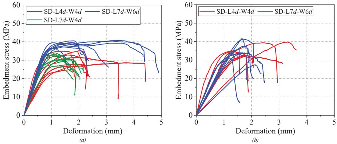
Figure 4. Embedment stress-deformation curves for: (a) smooth steel dowels and (b) DW dowels
