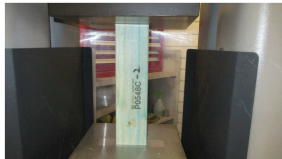
Figure 1. Test setup for measuring longitudinal compression strength.
