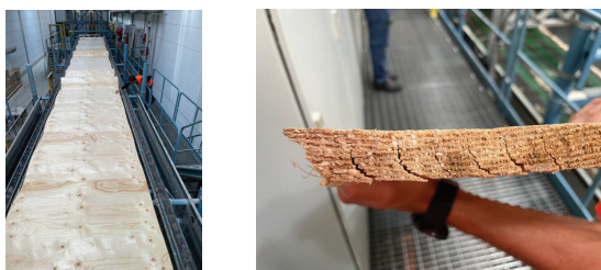
Figure 2: Impressions of the peeling process: (left) TPP strip after the lathe; (right) part of 20 mm thick TPP.
